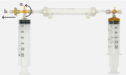
Step 11 a. Compress the air filter-side syringe, close the stopcock. b. Remove the air filter cap.
