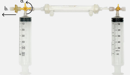
Step 11 a. Compress the air filter-side syringe, close the stopcock. b. Remove the air filter cap.
