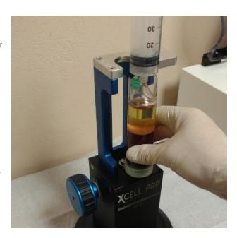
5. Gently turn the Knob counter-clockwise until the Concentrating Device touches the Top Plate.
