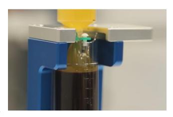
8. Detach the 60cc Syringe and cap using the provided Luer Lock Universal Cap and set aside.
