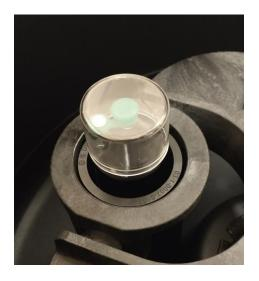
6. Close the lid and secure the lock by rotating clockwise to the vertical position as seen below.
