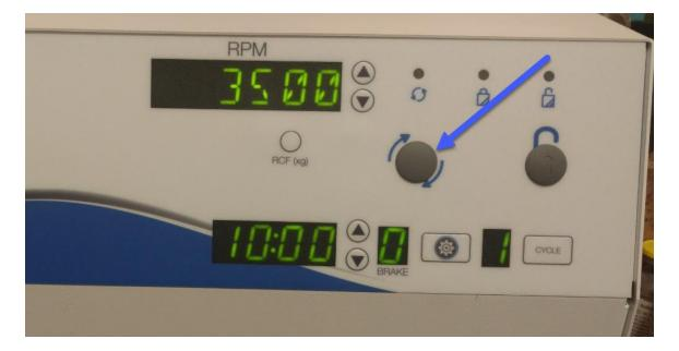
When the cycle is complete a tone will sound. Press the unlock button and open the lid. It is advisable to remove the Apex insert first, then remove the sample.
