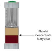
After spin, carefully remove **XCELL** concentrating device from the centrifuge. Remove the caps from Step 4.
