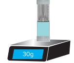
Secure the green silicone cap to the concentrating device cap. Match counterbalance to +/- 1.0g of concentrating device. Step 8:
